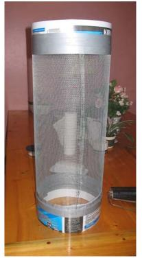
**Step 3:** Use the 24 gage wire to lace up the hardware cloth making a tight weave. You may have to double back to get a tight seam.
