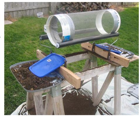
Grasp the top of the cylinder and pull down towards yourself and let it roll. One end of the harvester may need to be elevated so the material travels out the opposite end it is loaded. Make sure you have a container to catch the material larger than the screen. This can be mixed back into the worm bin and usually contains many worm eggs and unprocessed worm bedding.
