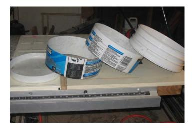
**Step 1:** The bucket was sectioned into two, four inch segments. The top and bottom were not used in this project. Please remember to use proper personal protective equipment and read your owners manuals for proper tool usage.
