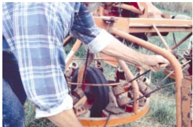
Slide 10. Adjusting the tedder. The tedder is adjusted from spreading the mowed grass to making a windrow.
