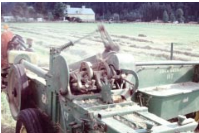
Slide 15. Proper adjustment of knotters and plunger will increase bale production per hour.
